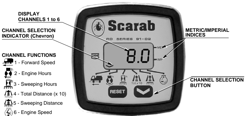
Fig. 15 The RDS Sweeper Monitor
