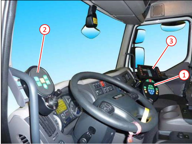
Main controller, operator screen and auxiliary controller
