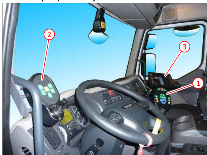
Main controller, operator screen and auxiliary controller
