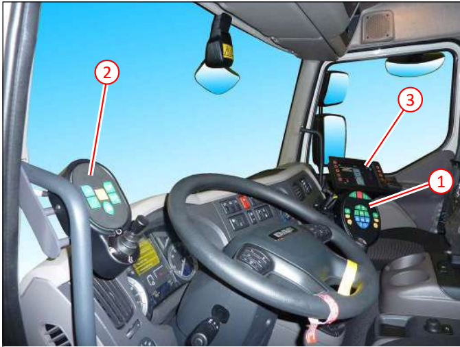
Main controller, operator screen and auxiliary controller
