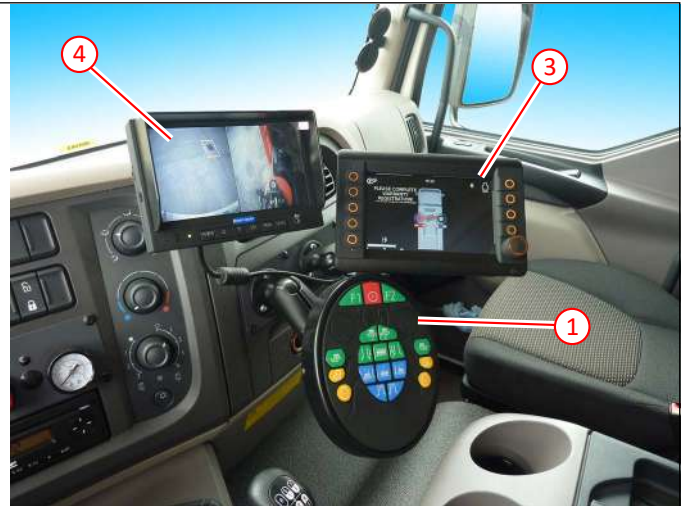
Main controller, operator screen and extra camera screen
