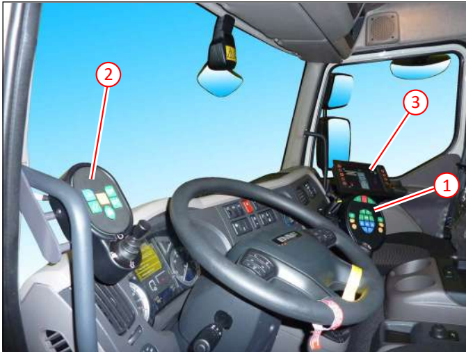
Main controller, operator screen and auxiliary controller
