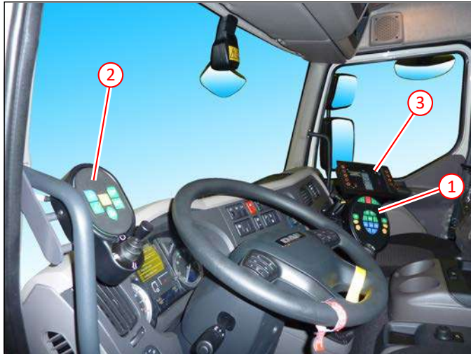
Main controller, operator screen and auxiliary controller
