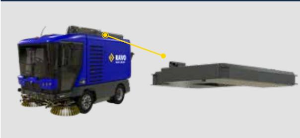
> An extra roof mounted 420-litre tank will give the sweeper a class leading total water capacity of over 950 litres without taking hopper space away. This enables a longer operating time between water refills, keeping the sweeper on the streets and on the go.
