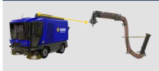
> The powerful RAVO wanderhose, now with hydraulic support, ideal for sucking leaves, emptying gullies and collecting debris from bins. It is supported by a hydraulic cylinder to lower or raise the hose making operation easy for the operator.
