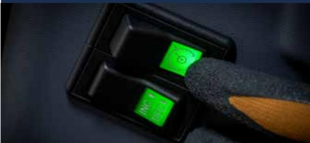
> Fully concentrate on the sweeping job by engaging cruise control in sweep mode. The cruise control mode allows the RAVO to sweep with a constant speed ideal for long straight roads.
