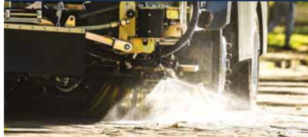
> Sweep up to 2.5 times longer with water being circulated from the hopper to the suction nozzle and back again, meaning that fresh water is only needed for the nozzles on the brushes. As a bonus, the water recycling system, which is easy to clean, suppresses dust emissions as well.
