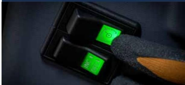
> Fully concentrate on the sweeping job by engaging cruise control in sweep mode. The cruise control mode allows the RAVO to sweep with a constant speed ideal for long straight roads.
