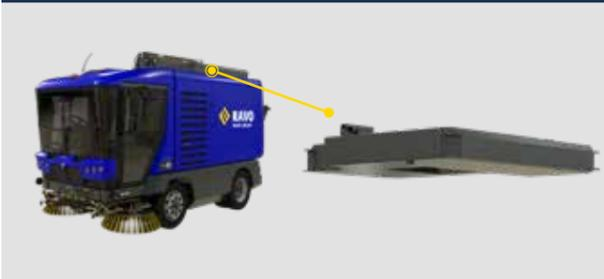
> An extra roof mounted 420-litre tank will give the sweeper a class leading total water capacity of over 950 litres without taking hopper space away. This enables a longer operating time between water refills, keeping the sweeper on the streets and on the go.
