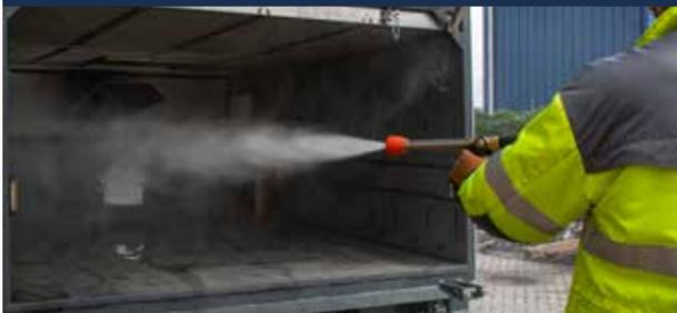
> The new spray gun now has two spray settings: a very powerful jet stream, and a wide-spread fan pattern that covers a larger area with greater efficiency. With this new high-pressure spray gun, operators can quickly and easily clean the sweeper and street furniture like bins and bus stops.
