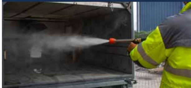
> The new spray gun now has two spray settings: a very powerful jet stream, and a wide-spread fan pattern that covers a larger area with greater efficiency. With this new high-pressure spray gun, operators can quickly and easily clean the sweeper and street furniture like bins and bus stops.
