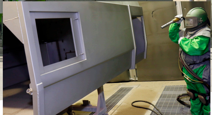
Shot blasting the hopper's stainless steel body
