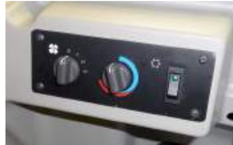
Cab heater controls with air conditioning
