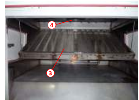
Screen in lowered position ready for cleaning
