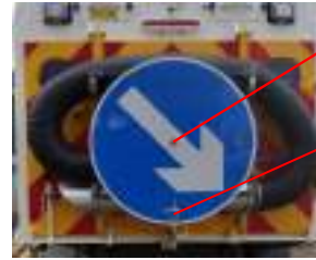
Traffic Sign Attached To Wander Hose Stowage Brackets
